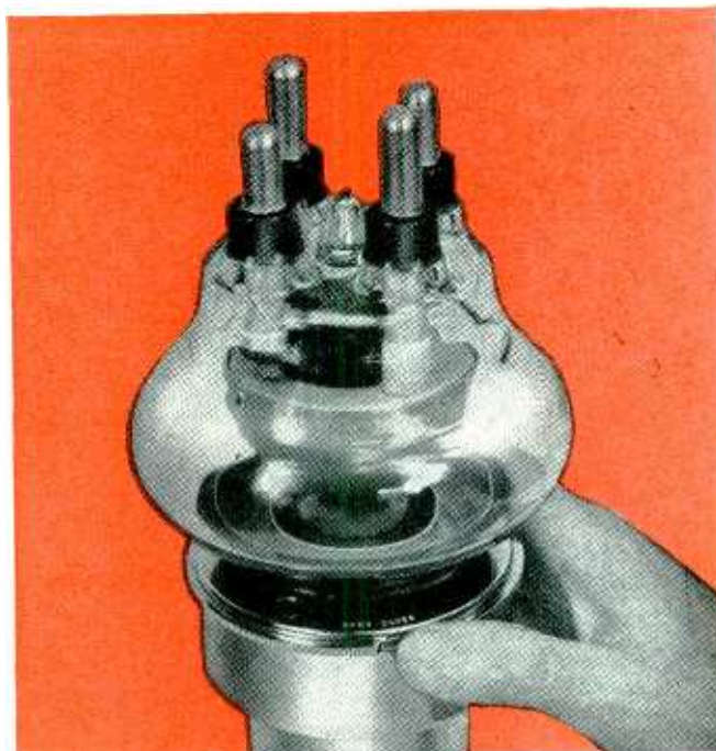
MACHLETT AUTOMATIC SEAL WATER JACKET.* No tools needed to open and close this new jacket. No worry about tube breakage or water leakage. Jacket cannot be opened unless water pressure is off, nor closed unless tube is properly seated. Your hand opens and closes a perfectly safe seal with just a single twist.
