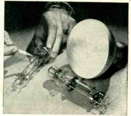
Westinghouse Sun Lamp uses "Z" Nickel springs to support quartz tube inside the lamp. Temperatures up to 750°.
