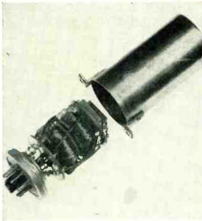
FIG. 3—Plug-in oscillator tank circuit using the sealed construction
